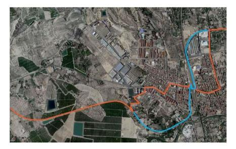
Campos del Río: Work has been done on two sections in this municipality. In the area around La Casilla, to the north east of the town, a long (900 metre) section of the original railway line has been incorporated, reducing the detour that previously been signposted by more than 850 metres.
